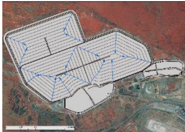
Figure 1 The TSF landform construction design contours
