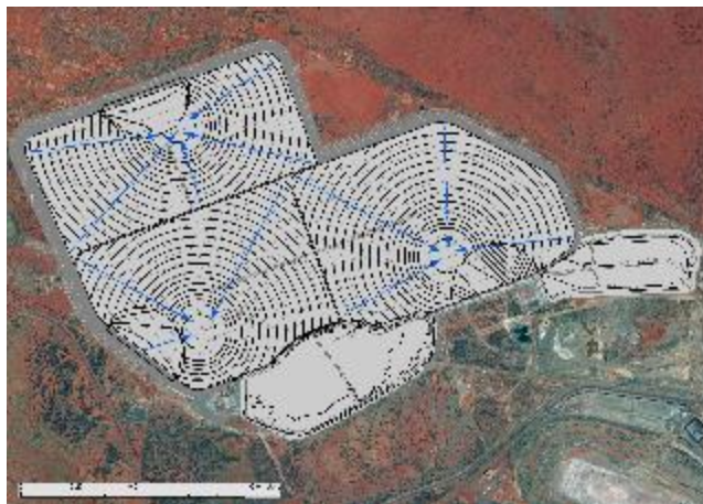
Figure 4 Ideal tailings beach surface contours, matching the contours of the final landform
